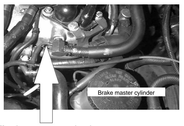
Mount boost gauge pressure tube and "T" fitting to this port on the drivers side rear of the engine.
